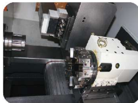
➤ Hydraulic Turret + Cross Drilling Device
