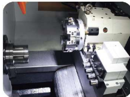
➤ Hydraulic Turret + Face Drilling Device
